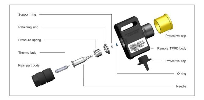
The Remote TPRD (Thermal Pressure Relief Device) 023564-F is used to secure gas storage tanks in the event of a fire by ensuring rapid and spatially targeted degassing at elevated temperatures whilst preventing the tanks from bursting.
