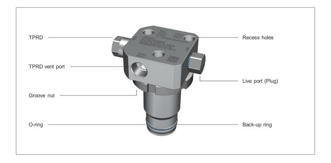
The End Plug TPRD (Thermal **P**ressure **R**elief **D**evice) is used to secure hydrogen gas storage tanks in the event of a fire by ensuring rapid and spatially targeted degassing at elevated temperatures whilst preventing the tanks from bursting.
